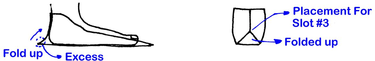
Figure 3 Determining the Heel Excess
